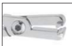
GS-3070 Detailing step plier double-sided offset beak permits bayonet bends. Creates right hand or left hand step-up or stepdown at 1/2, 3/4, or 1mm increments.
